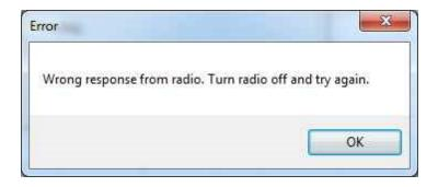
This error is VERY common in the radios that use the 2-pin plug into the mic jack. It is resolved by pushing the cable again... a little harder so that it seats completely into the mic jack.
