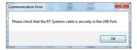
The USB-57A programming cable or the original RT Systems serial programming cable with the RTS-03 USB to serial adapter are the only two cable configurations that will be recognized by the FT-50 Version 4 programmer.
