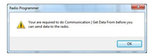
This indicates that you have not read the configuration of the radio into the programmer.
