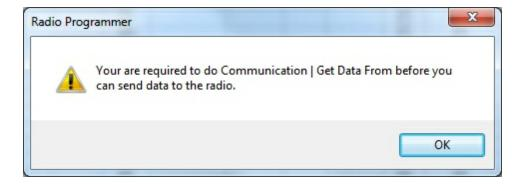
This indicates that you have not read the configuration of the radio into the programmer.
