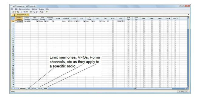
Click a tab. A screen opens with the details that can be entered for these radio functions. You can work with the radio without ever using these tabs. There are default values on these screens that never need to be changed. Make changes for your special activities when you plan to use one of these functions of the radio.
