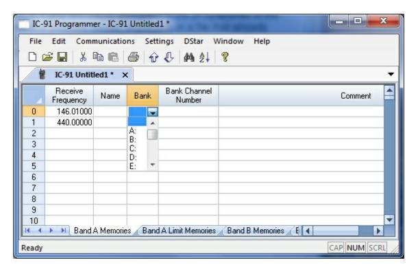
Receive Frequency, Name (memory channel name), Bank, and Bank Channel Number remain on the screen eliminating the need to scroll from left to right accessing these columns.
