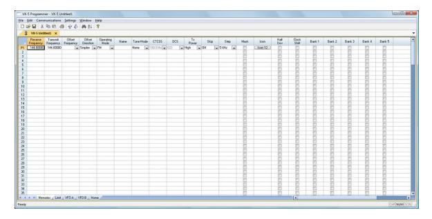
Note: The default file contains memory channel information on several of the screens. This information is needed by the radio to "fill spaces in its little brain". You can change the default entries that you see; but anything that is completed in the default file cannot be left blank. The Programmer will help you with this. If information is required, it will warn you when it is missing.
