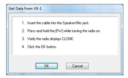
**2).** Once the radio displays CLONE, click the OK on the computer screen. A second window opens with the last instruction for the process.
