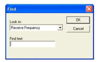
Select the field to be searched (i.e., Receive frequency, Transmit frequency, etc.)
