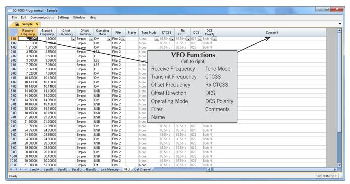
**VFO** The program makes available the same VFO's as in the radio. Remember these are not real memory channels since the details are lost as soon as you tune the radio manually. There is no one button recall for these. You do not need to program into VFO before programming details into a memory channel.\*
