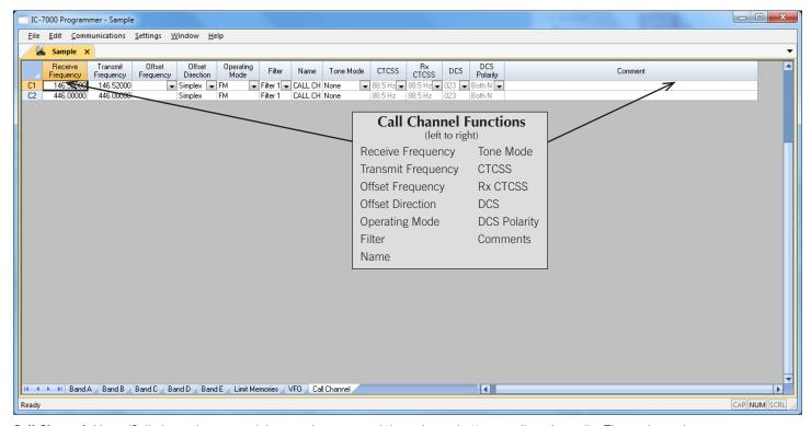
**Call Channel** Home/Call channels are special memories accessed through one button recall on the radio. These channels are preprogrammed in the radio and while the frequency can be changed to another within the band, they cannot be left blank.
