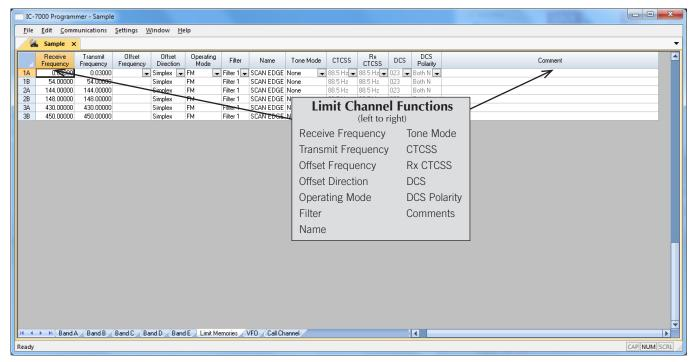
**Limit Memories** Limit Memories are used by the radio for Programmed Scan Operations. Program the same details for Limit Memories as for regular memory channels.\*
