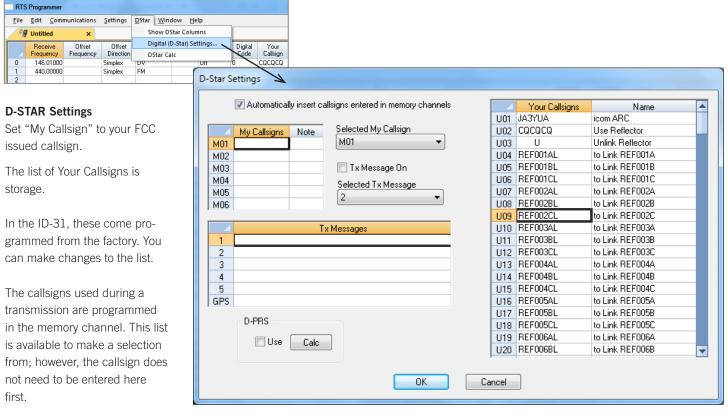
Tx messages, name/location/equipment details, etc., scroll on the radio receiving your call. Be sure to turn on the Tx message with the checkbox.
